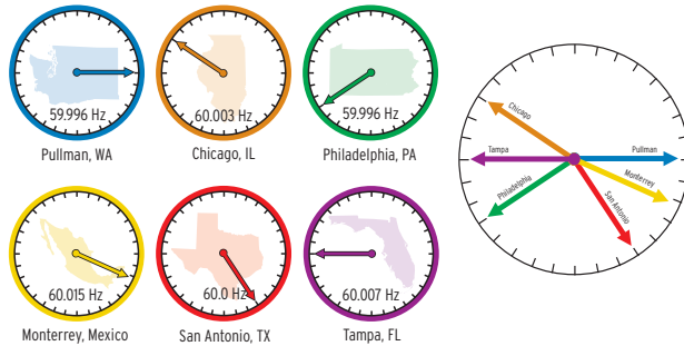
Figure 11 View of System Angle at Multiple Locations
