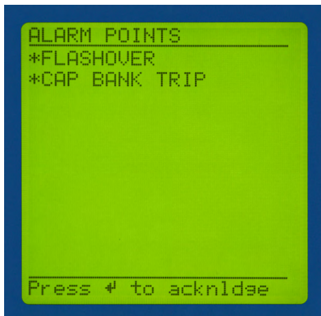
Figure 12 Sample Alarm Points Screen
