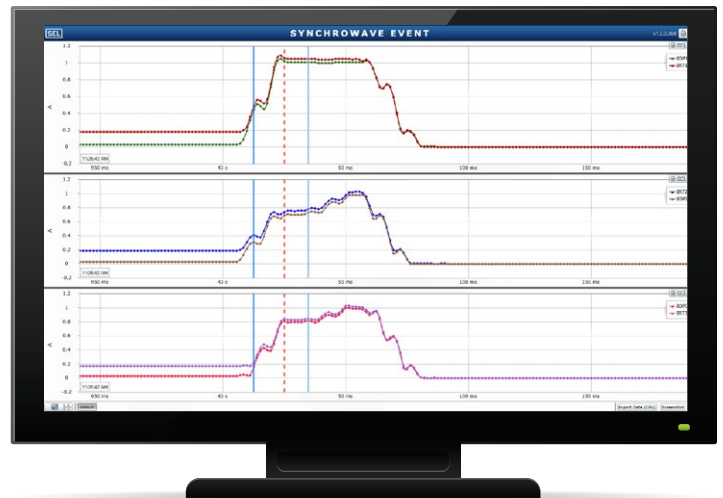
SYNCHROWAVE Event displays individual operate and restraint currents for three different protection zones.
