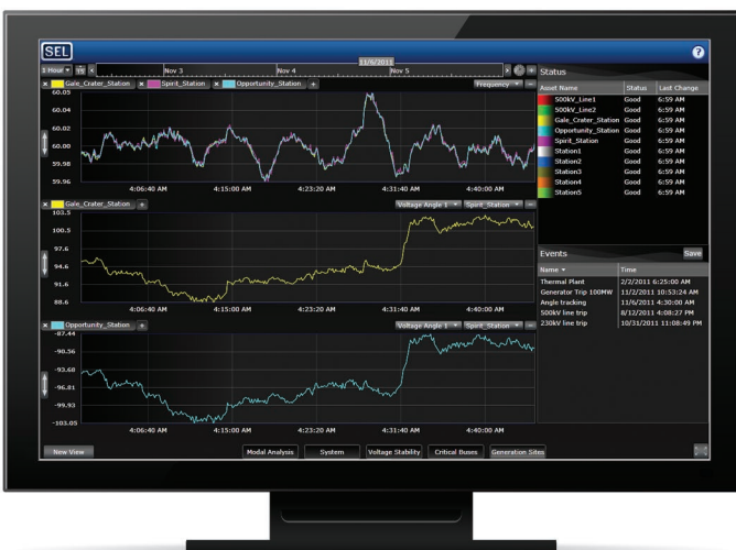
SEL-5078-2 SYNCHROWAVE Central Software provides visualization and analysis of power system operating conditions.
